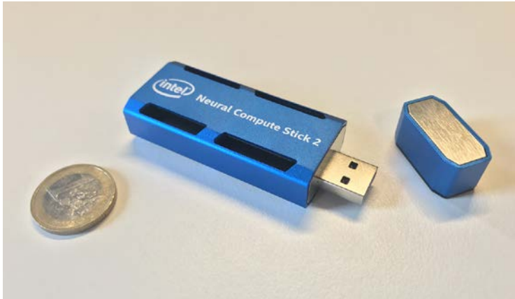
Рис. 15.3. Intel Neural Compute Stick 2
