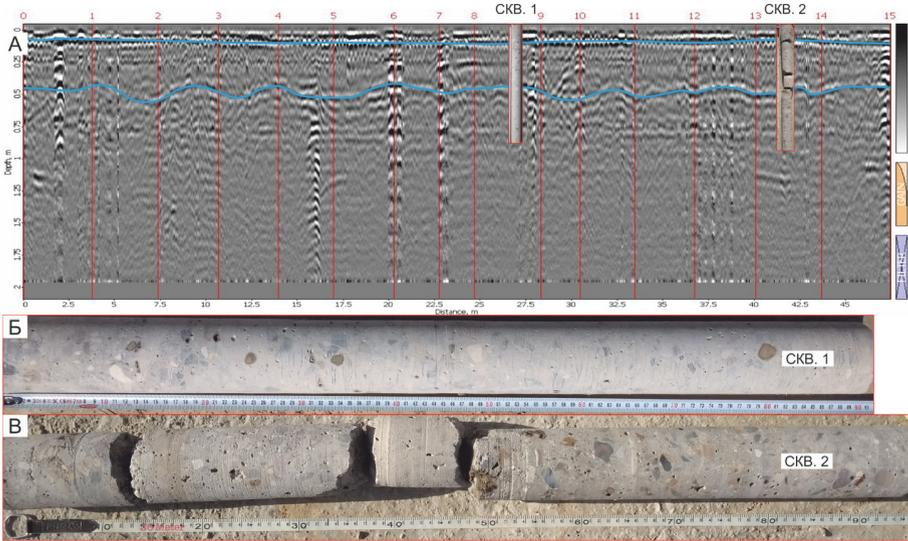
**Fig. 1.** Determination of cold contact boundaries: A - interpreted radarogram, B—core from hole 1, C—core from hole 2.
