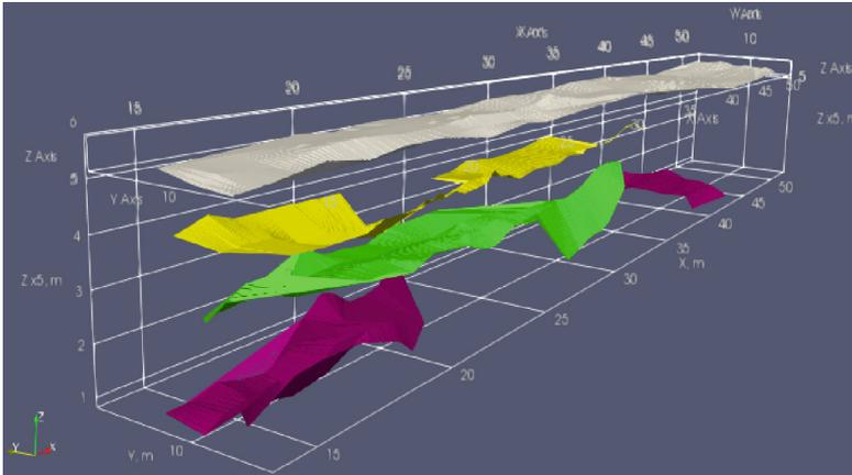
**Fig. 7.** A3D visualization of the roof slab with cold joints. Violet, first boundary; green, second boundary; Yellow, third boundary; grey, top surface of the roof slab
