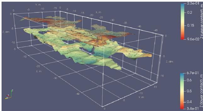
**Fig. 3.** Depth maps of the surfaces of the first (A) and second (B) cold contacts (independent color scales).
