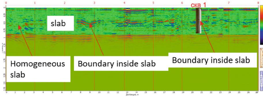
**Fig. 4.** A typical radarogram showing the boundaries in the structure of the foundation plate.
