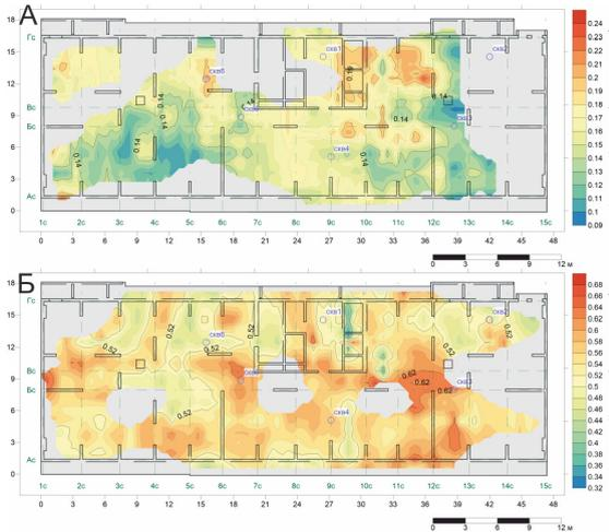
**Fig. 2.** Depth maps of the surfaces of the first (A) and second (B) cold contacts (independent color scales).
